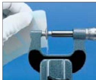
169-101 with holohedral measuring surfaces
