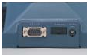
DIGIMATIC- and RS-232 C data output port (standard)
