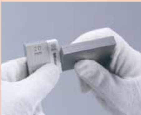
Sample application Steel and ceramic gauge blocks used together.
